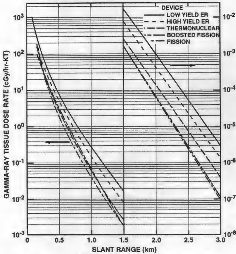
Figure 8.26. Gamma-Ray Dose Rate per Kiloton Yield at 1 hour Versus Slant Range From Neutron Activation of European Soil for Various Nuclear Weapon Types.
